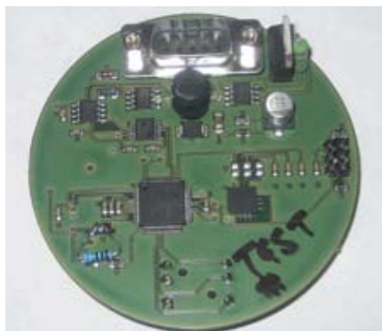
Above: Rear of the production prototype circuit board showing processor, power supply and interface electronics. Below: Front showing display and joystick control.
