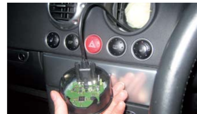
With the circuit board mounted in a modified air vent, installation is straightforward. The cable is threaded down to the OBDII diagnostics port for semi-permanent connection.
