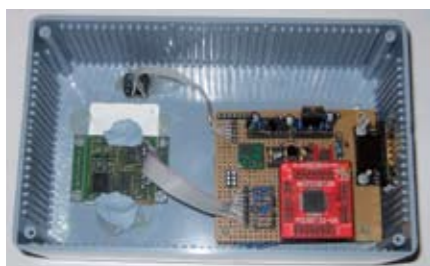
Early standalone prototype, left, and processor development board for PC-based software development kit, right.
