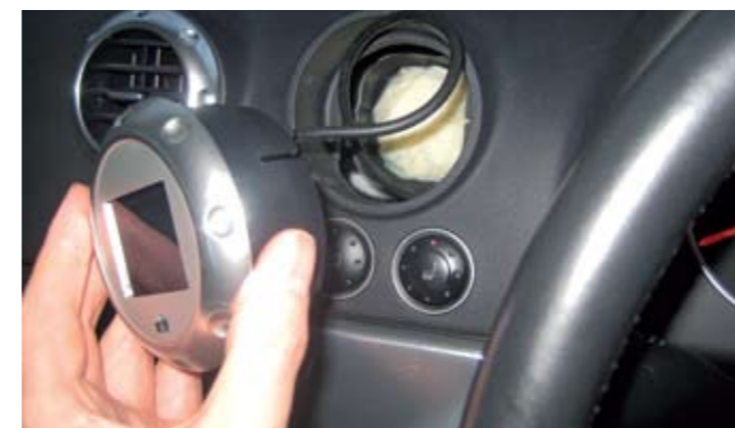
With the circuit board mounted in a modified air vent, installation is straightforward. The cable is threaded down to the OBDII diagnostics port for semi-permanent connection.
