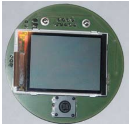
Above: Rear of the production prototype circuit board showing processor, power supply and interface electronics. Below: Front showing display and joystick control.
